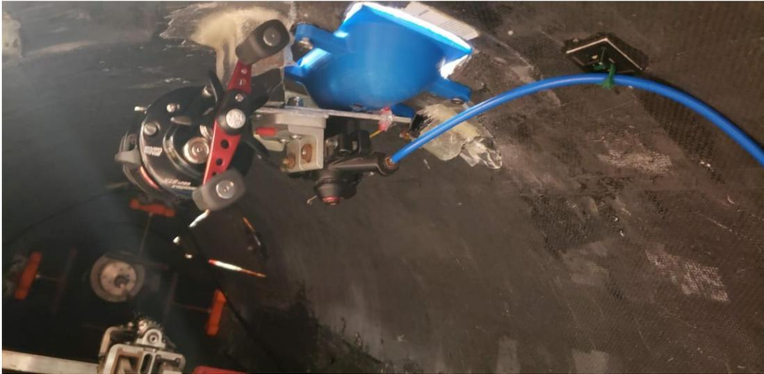
*Figure 7: The buoy release mechanism in Phantom 8*
