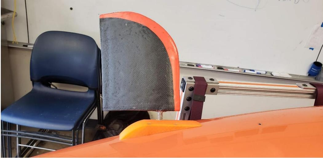
*Figure 6: The control surface on the top of Phantom 8*
