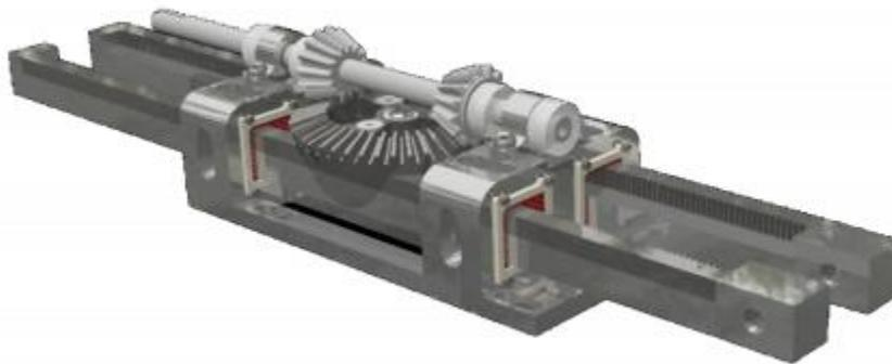
*Figure 1: A rendering of the primary gearbox in Phantom 8*
