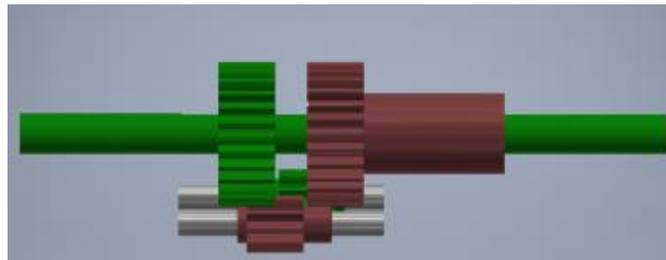
Figure 3: The green and red components rotate opposite of each other to produce contra-rotation
