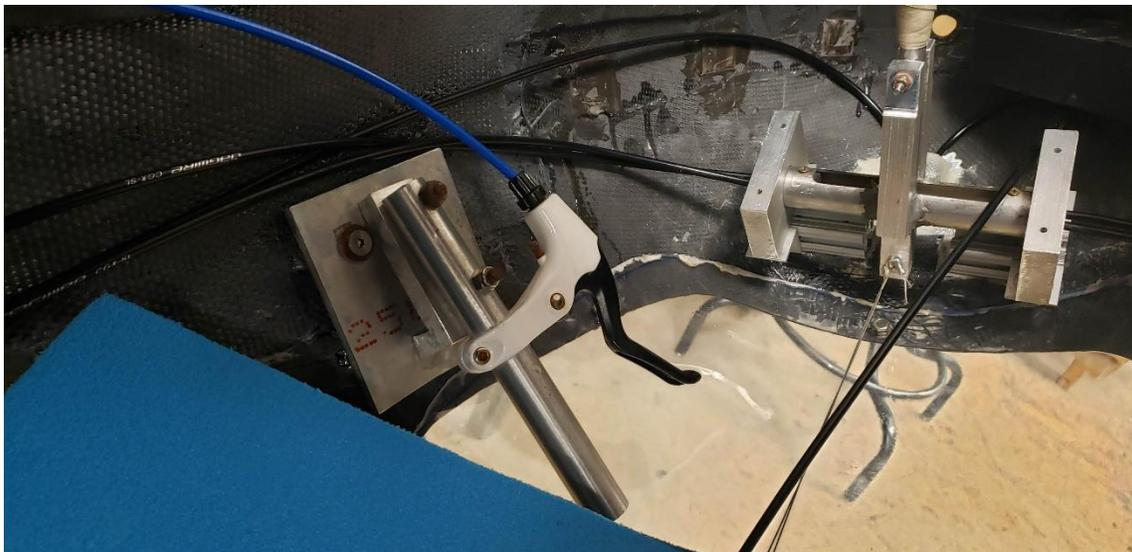
*Figure 8: The dead-man switch in Phantom 8*
