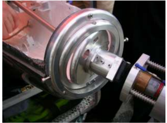
Figure 16. Vectored thrust system with a view of the variable pitch system attached.
