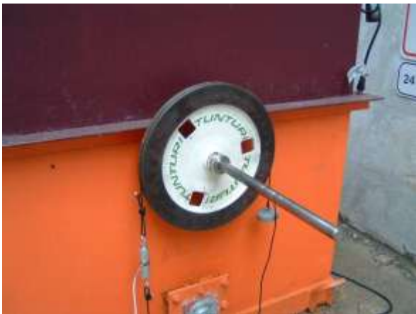
Figure 8. The fly wheel and brake used for measuring the torque produced by the pilot.
