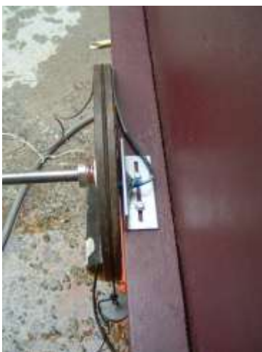
Figure 9. The Hall effect transducer.
