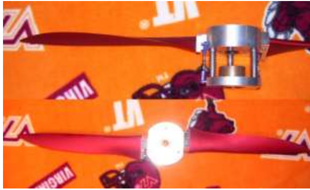
Figure 14. Completed, anodized blades in variable pitch hub.
