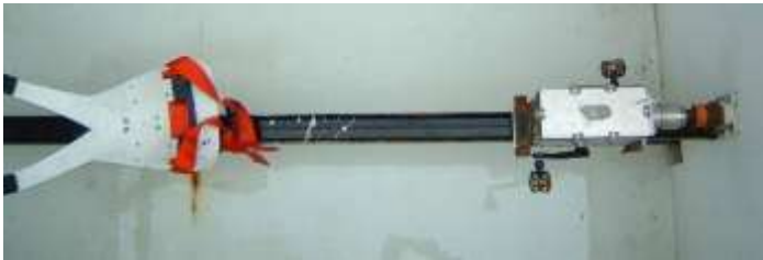
Figure 7. The pilot harness and gear box mounted inside the test tank.
