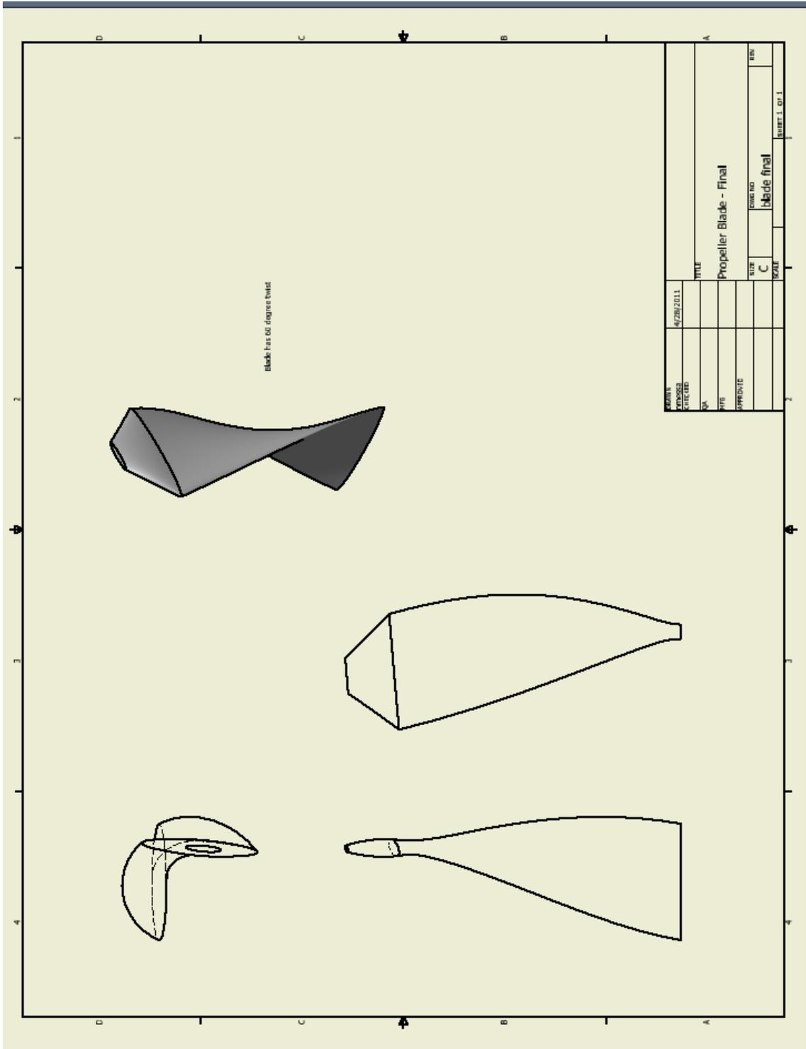
Figure 6 Propeller Blade with 60 degree twist
