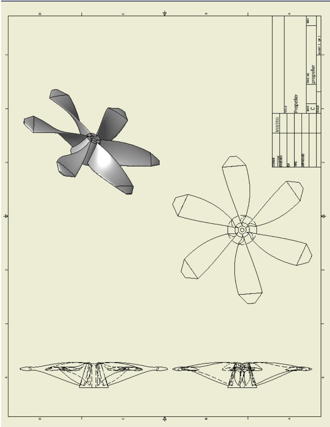
**Figure 3 Propeller Assembled**
