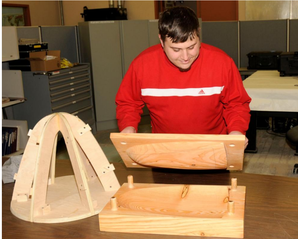
Figure 11-Mold Designer Demonstrates Bow Dome Viewing Pane Mold
