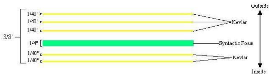
Figure 7: Hull Layers and Thicknesses
