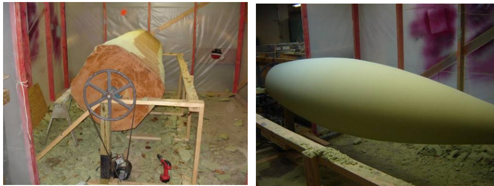
Figure 8: Foam Block Lathing Set-up and Final Hull Form
