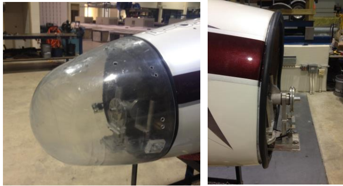
Figure 9: Nose Cone and Weather-Stripping on Rim
