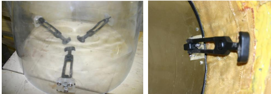
Figure 10: Rubber-Tension Latches and Connection to Plastic Notch
