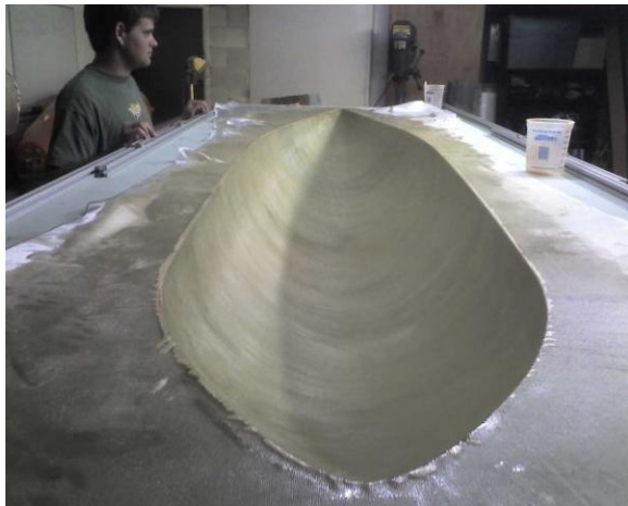
The female foam mold of Swamp Thing II's hull
