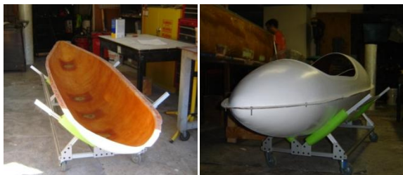
A single half-mold and two half-molds joined together are shown.
