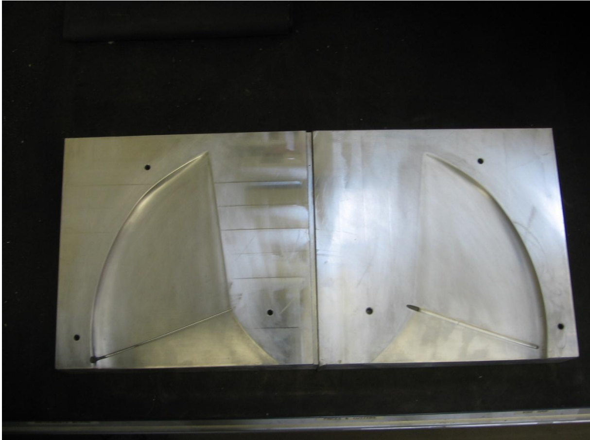
Figure 45- Fins machined mold
