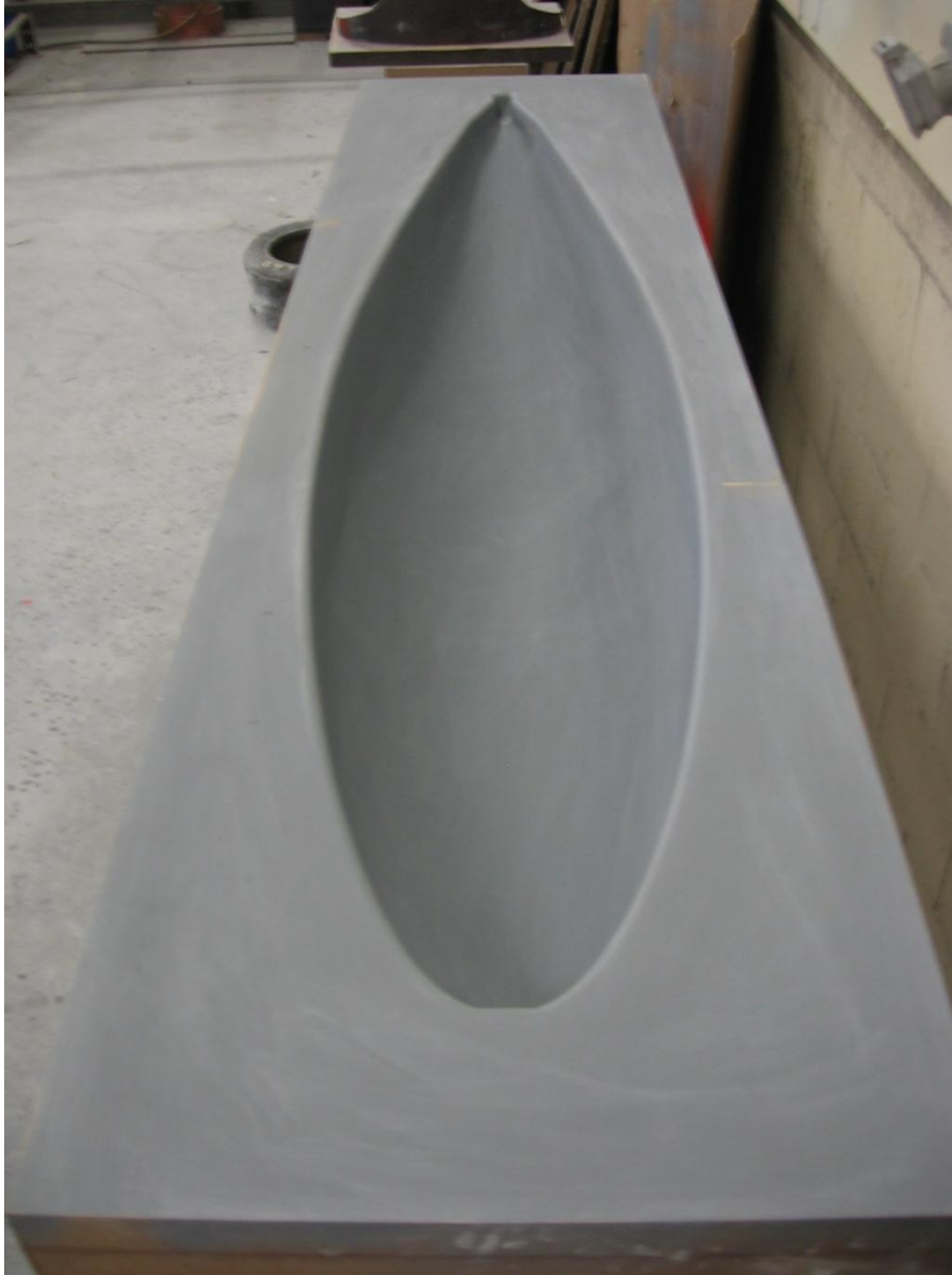
Figure 50- Painted mold of the hull
