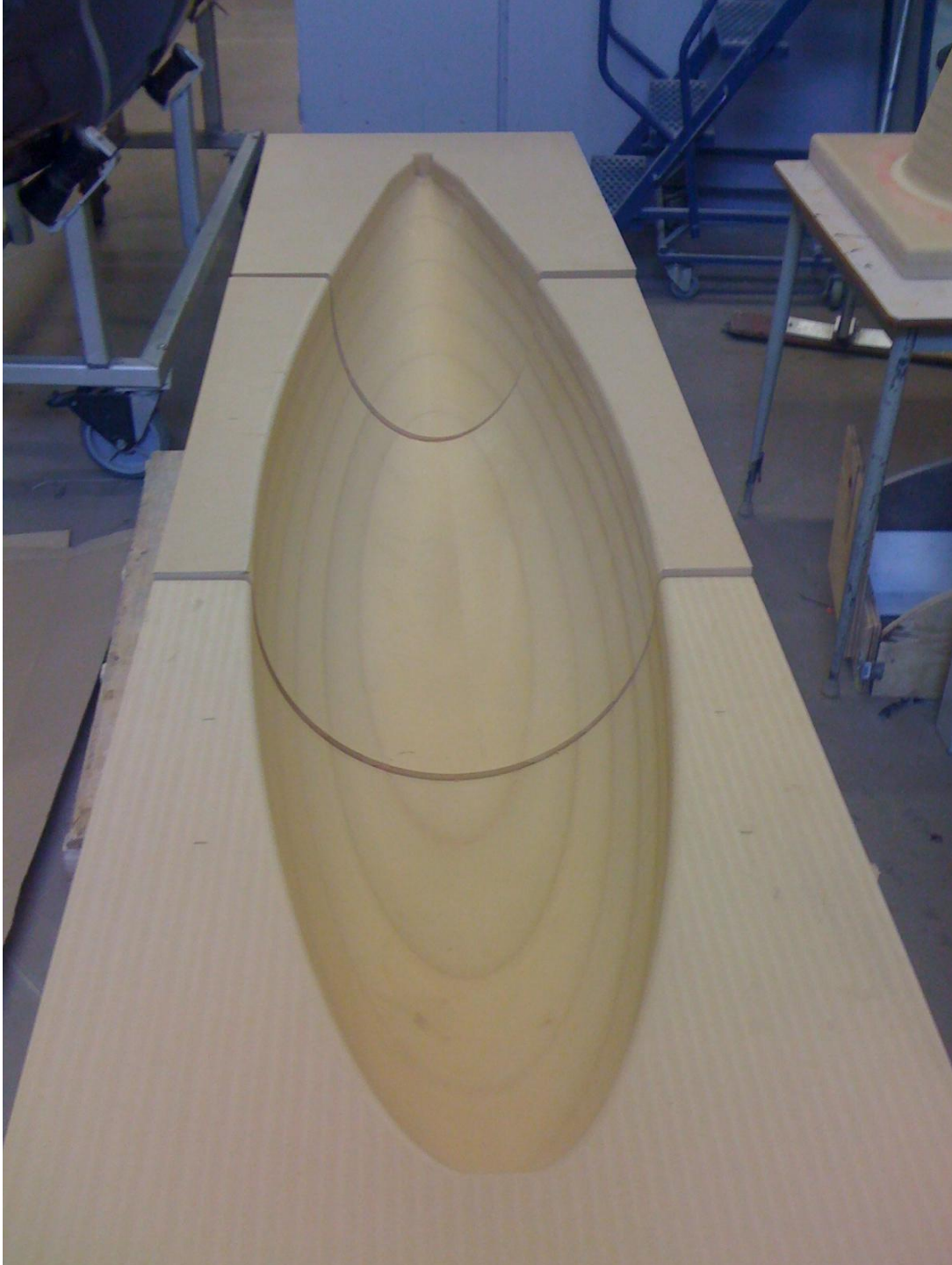
Figure 48-Machined mold of the hull
