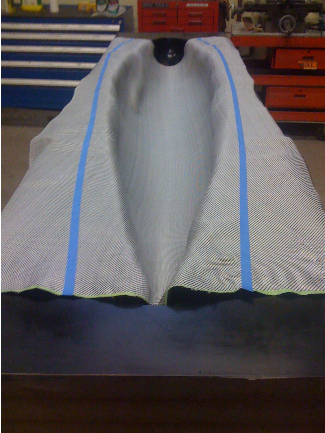
Figure 52- Placing the carbon fiber in the mold
