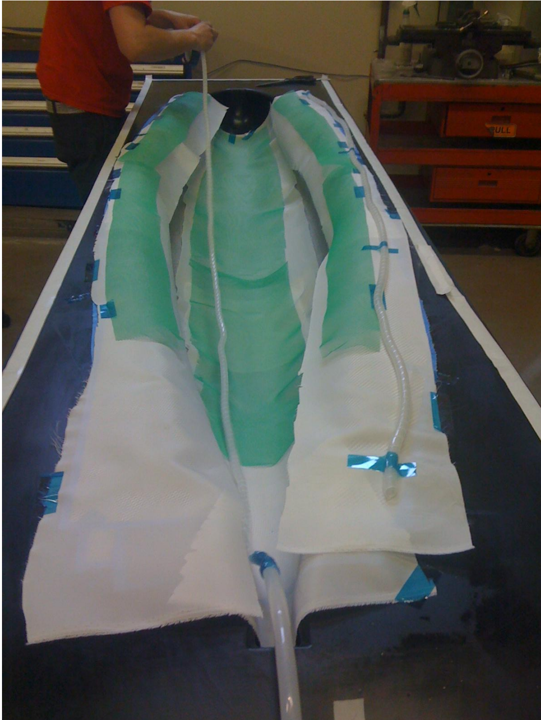
Figure 54-Placing the peel ply and the tubing
