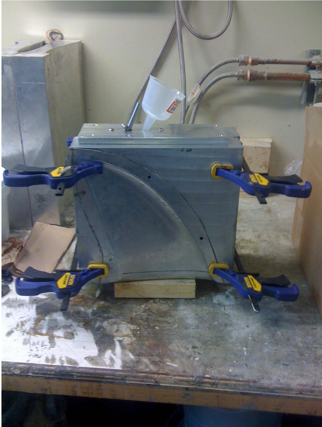
Figure 46-The molding of the fins
