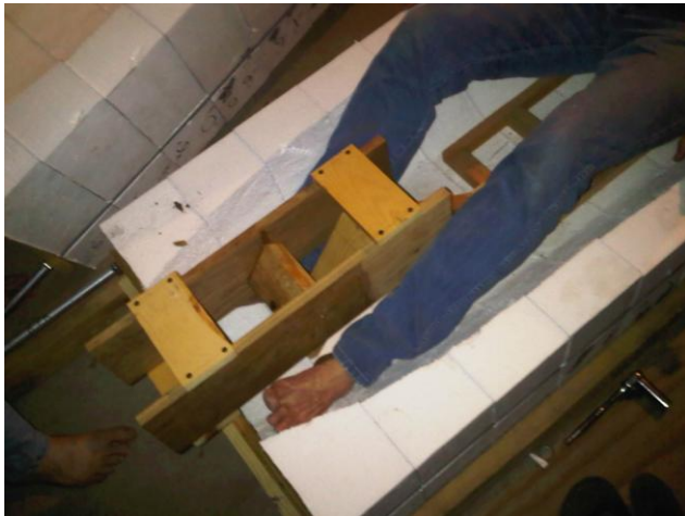
Figure 9b – Testing Placement of a Mockup Linear Drive for Placement and Relative Leg Angle
