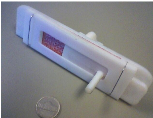
Figure 10 – Linear Drive Proof of Concept Prototype – 1/4 Scale
