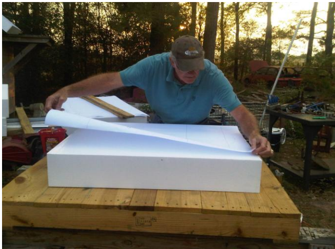
Figure 7a – Applying Computer Generated Sections on 6" Foam Blocks
