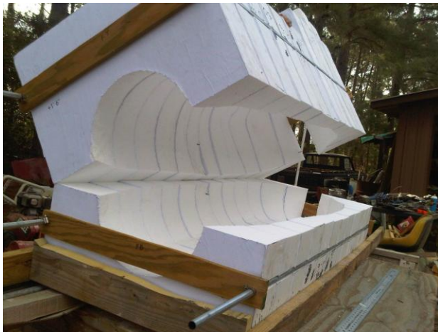
Figure 7d – Hull Split Horizontally Ready for Interior Space Study
