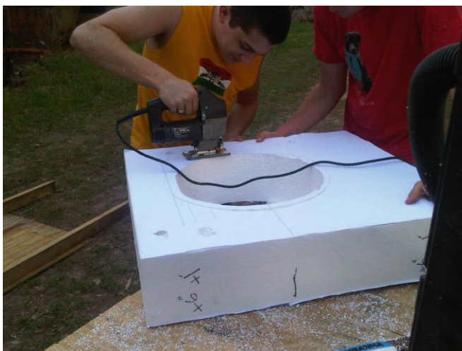
Figure 7b – Cutting Foam Blocks to Pattern
