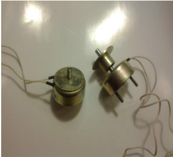
The two DC solenoids used in the dead-man system's configuration.
